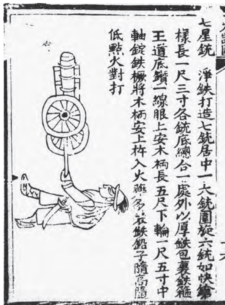
A seven-barreled organ gun with two auxiliary guns by its side on a two-wheeled carriage from the Huolongjing . Source: Wikimedia Commons at https://tinyurl.com/y67evkyy .
