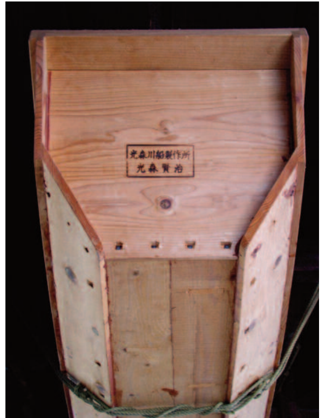
Figure 1. View of the sasabune stern. Note how the lower hull planks extend slightly below the base of the boat. Exposed fasteners are visible along the base of the transom and hull planking. Photo by Michelle Damian.
