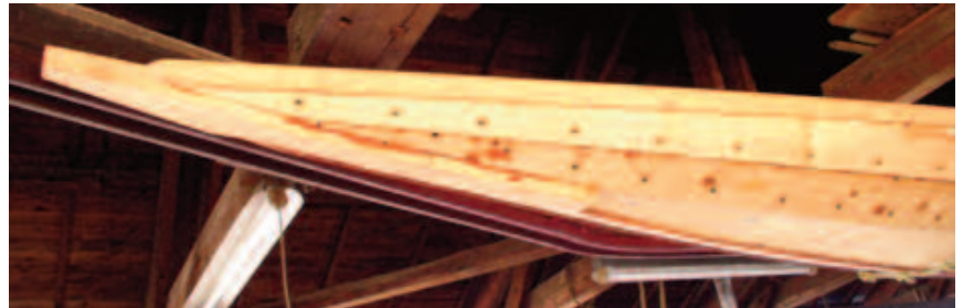
Figure 2 Side view of the sasabune bow, showing the hull planks meeting the stempost. Photo by Michelle Damian.
