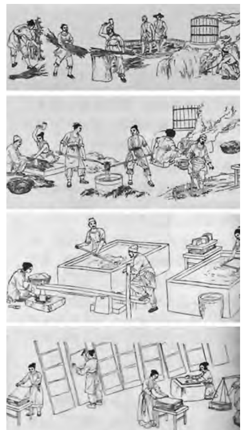
The woodblock prints show some of the six major stages in papermaking, recorded in a seventeenth-century book The Exploitation of the Works of Nature .
